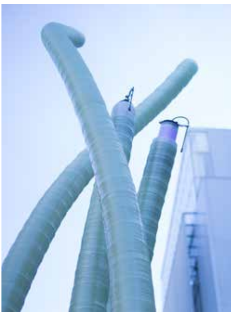
Fiberbots, robotic fabrication of structure in progress. The Mediated Matter Group. MIT Media Lab. 2018.
